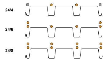
**Note:** o indicates location of arc spot weld, power actuated fastener, or screw as indicated in the load tables. indicates location of arc seam weld, power actuated fastener, or screw as indicated in the load tables.
